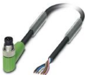
Sensor/actuator cable, 6-position, PUR halogen-free, black-gray RAL 7021, Plug angled M8, on free cable end, cable length: 3 m
