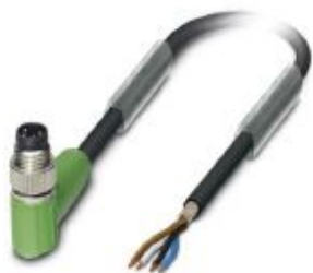
Sensor/actuator cable, 4-position, PUR halogen-free, black-gray RAL 7021, shielded, Plug angled M8, on free cable end, cable length: 3 m
