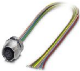
Sensor/Actuator flush-type socket, 8-pos., M12, A-coded, front/screw mounting with Pg9 thread, with 0.5 m TPE litz wire, 8x 0.25 mm 2
