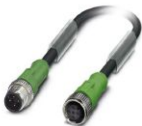
Sensor/actuator cable, 4-position, PUR, black-gray RAL 7021, Plug straight M12, coding: A, on Socket straight M12, coding: A, cable length: 1 m
