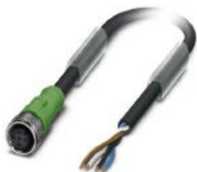
Sensor/actuator cable, 4-position, PUR, black-gray RAL 7021, free cable end, on Socket straight M12, coding: A, cable length: 2 m
