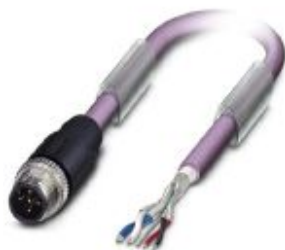
Bus system cable, CANopen®, DeviceNet™, 5-position, PUR halogen-free, violet RAL 4001, shielded, Plug straight M12, coding: A, on free cable end, cable length: 15 m
