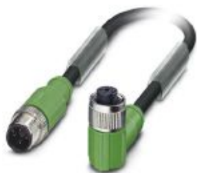
Sensor/actuator cable, 4-position, PUR halogen-free, black-gray RAL 7021, shielded, Plug straight M12, coding: A, on Socket angled M12, coding: A, cable length: 3 m
