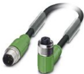
Sensor/actuator cable, 3-position, PUR halogen-free, black-gray RAL 7021, shielded, Plug straight M12, coding: A, on Socket angled M12, coding: A, cable length: 3 m
