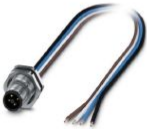
Flush-type connector, Power, 4-position, Plug, M12, T power, Rear mounting, M16 x 1.5, Individual wires, cable length: 0.25 m, 1.31 mm 2 , UL/cUL stranded hook-up wire
