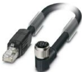
Assembled VARAN cable, shielded, stranded, black, angled M12 socket, SPEEDCON, 6-pos. to RJ45 plug/ IP20, QUICKON, length: 2 m
