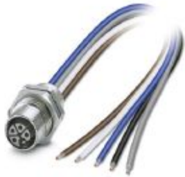
Flush-type connector, Power, 5-position, Socket, M12, L - Power, Rear mounting, M16 x 1.5, Individual wires, cable length: 0.2 m, 2.50 mm², PEX litz wire
