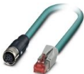
Network cable, Ethernet CAT5 (1 Gbps), 8-position, PUR, water blue RAL 5021, shielded, Plug straight RJ45 / IP20, cable length: 5.9 m
