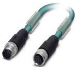
Bus system cable, 8-position, PUR, water blue RAL 5021, Plug straight M12, coding: A, on Socket straight M12, coding: A, cable length: 40 m
