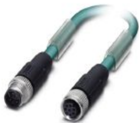
Bus system cable, 8-position, PUR, water blue RAL 5021, Plug straight M12, coding: A, on Socket straight M12, coding: A, cable length: 15 m
