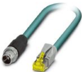
Network cable, Ethernet CAT6 A (10 Gbps), 8-position, PUR, water blue RAL 5021, shielded, cable length: 20 m, Customer version
