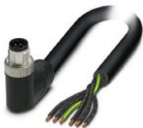
Power cable, 6-position, PVC, black-gray RAL 7021, Plug angled M12, coding: M, on free cable end, cable length: 3 m, For AC current up to 8 A/690 V
