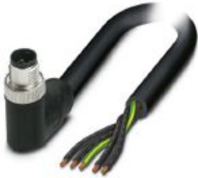
Power cable, 5-position, PUR halogen-free, black-gray RAL 7021, Plug angled M12, coding: K, on free cable end, cable length: 3 m, for AC current up to 16 A/690 V
