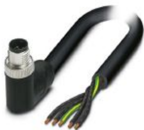
Power cable, 5-position, PUR halogen-free, black-gray RAL 7021, Plug angled M12, coding: K, on free cable end, cable length: 1.5 m, for AC current up to 16 A/690 V
