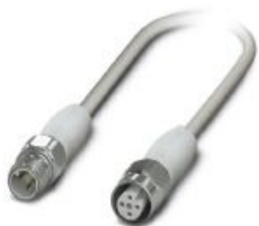
Sensor/actuator cable, 4-position, PP-EPDM halogen-free, gray RAL 7035, shielded, Plug straight M12, coding: A, on Socket straight M12, coding: A, cable length: 0.6 m, Hygienic design, with high-grade steel knurl
