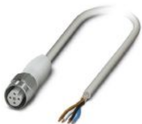
Sensor/actuator cable, 4-position, PP-EPDM halogen-free, gray RAL 7035, shielded, free cable end, on Socket straight M12, coding: A, cable length: 3 m, Hygienic design, with high-grade steel knurl
