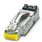
RJ45 connector, IP20, CAT6<sub>A</sub>, 8-pos., with IDC fast connection technology, for AWG 26 - 24 1-wire, 7-wire, and 19-wire conductors
