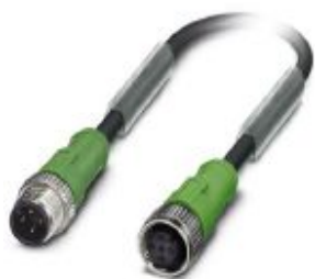
Sensor/actuator cable, 4-position, Variable cable type, Plug straight M12, coding: A, on Socket straight M12, coding: A, cable length: Free input (0.2 ... 40.0 m)
