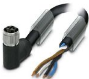
Power cable, 4-position, PVC, black-gray RAL 7021, free cable end, on Socket angled M12, coding: T, cable length: 1 m, For direct current up to 12 A/63 V
