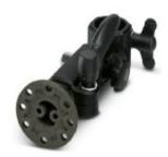
140.5 mm housing attachment, for max. load 10 kg, with ball joint and fastening plate 60 mm, pivotable in 15° increments, for 30 mm wall/profile bracket, material: black glass-fiber reinforced polycarbonate PC, and black anodized aluminum, 342 g
