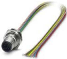
Sensor/actuator flush-type plug, 12-pos., M12 SPEEDCON, rear/screw mounting with M16 thread, with 0.5 m TPE litz wire, 12 x 0.14 mm 2
