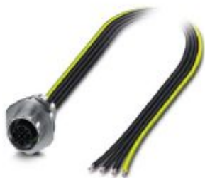
Flush-type connector, Power, 4-position, Socket, M12, S power, Front mounting, M16 x 1.5, Individual wires, UL/cUL stranded hook-up wire
