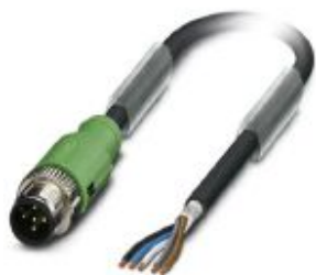
Sensor/actuator cable, 5-position, PUR halogen-free, black-gray RAL 7021, shielded, Plug straight M12 SPEEDCON, coding: A, on free cable end, cable length: 2 m
