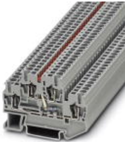
Component terminal block, connection method: Spring-cage connection, cross section: 0.08 mm² - 4 mm², AWG: 28 - 12, length: 67.5 mm, width: 5.2 mm, color: gray, mounting: NS 35/7,5, NS 35/15, DIN rail mounting
