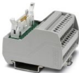
VARIOFACE module, with screw connection and flat-ribbon cable connector, for mounting on NS 35 rails, with pin strip and short and long locking latches for socket strips, 20-pos., with LED
