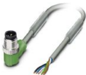
Sensor/actuator cable, 5-position, PUR halogen-free, resistant to welding sparks, highly flexible, gray RAL 7001, Plug angled M12, coding: A, on free cable end, cable length: 5 m, for robots and drag chains
