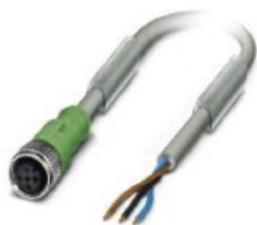
Sensor/actuator cable, 3-position, PUR halogen-free, resistant to welding sparks, highly flexible, gray RAL 7001, free cable end, on Socket straight M12, coding: A, cable length: 3 m, for robots and drag chains
