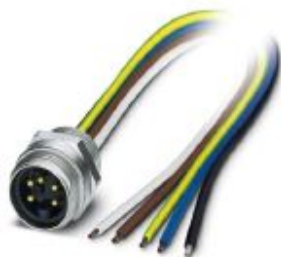
Sensor/actuator panel-mount connector, 5-pos., 7/8", front mounting with Pg13.5 thread, with 2.0 m PVC litz wire, 5 x 0.75 mm 2
