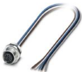
Sensor/actuator flush-type socket, 5-pos., M12, B-coded, front/screw mounting with Pg9 thread, with 0.5 m TPE litz wire, 5 x 0.34 mm², stainless steel version
