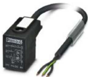
Sensor/actuator cable, 3-position, PUR halogen-free, black-gray RAL 7021, free cable end, on Valve connector BI (11 mm), with 1 LED, connected with Varistor, cable length: 3 m
