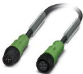
Sensor/actuator cable, 5-position, PUR halogen-free, black-gray RAL 7021, Plug straight M12, coding: A, on Socket straight M12, coding: A, cable length: 0.3 m, with plastic knurl
