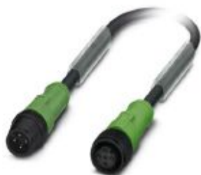
Sensor/actuator cable, 4-position, PUR halogen-free, black-gray RAL 7021, Plug straight M12, coding: A, on Socket straight M12, coding: A, cable length: 3 m, with plastic knurl
