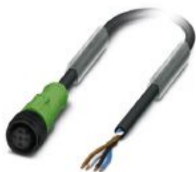
Sensor/actuator cable, 4-position, PUR halogen-free, black-gray RAL 7021, free cable end, on Socket straight M12, coding: A, cable length: 5 m, with plastic knurl
