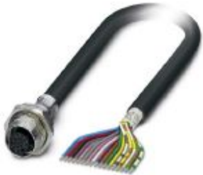
Flush-type socket, shielded, 17-pos., M12, A-coded, rear/screw mounting with M16 thread, with 1 m cable, 17 x 0.14 mm²
