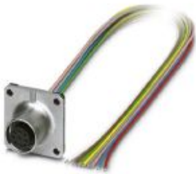
Sensor/actuator flush-type socket, 8-pos., M12, A-coded, front/square flange mounting, with 0.5 m TPE litz wire, 8 x 0.25 mm 2
