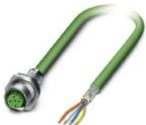
Bus system flush-type socket, PROFINET, 4-pos., M12, shielded, D-coded, SPEEDCON, rear/screw mounting with Pg9 thread, with 1.0 m bus cable, 2 x 2 x 0.34 mm 2
