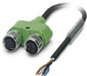
Sensor/actuator cable, 4-position, PUR halogen-free, black-gray RAL 7021, free cable end, on Socket straight M12 SPEEDCON, coding: A and Socket straight M12 SPEEDCON, coding: A, cable length: 1.5 m
