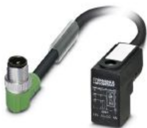
Sensor/actuator cable, 3-position, PUR halogen-free, black-gray RAL 7021, Plug angled M12 SPEEDCON, coding: A, on Valve connector C (8 mm), with 1 LED, connected with Z diode, cable length: 1.5 m
