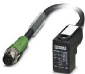
Sensor/actuator cable, 3-position, PUR halogen-free, black-gray RAL 7021, Plug straight M12 SPEEDCON, coding: A, on Valve connector C (8 mm), with 1 LED, connected with Z diode, cable length: 0.3 m
