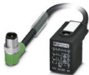
Sensor/actuator cable, 3-position, PUR halogen-free, black-gray RAL 7021, Plug angled M12 SPEEDCON, coding: A, on Valve connector B (10 mm), with 1 LED, connected with Z diode, cable length: 0.3 m
