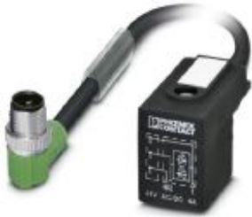
Sensor/actuator cable, 3-position, PUR halogen-free, black-gray RAL 7021, Plug angled M12 SPEEDCON, coding: A, on Valve connector BI (11 mm), with 1 LED, connected with Z diode, cable length: 0.3 m
