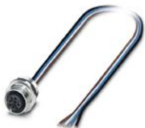
Bus system flush-type connector, FOUNDATION Fieldbus, socket, 4-pos., M12, A-coded, front/screw mounting with Pg9 thread, with 0.5 m TPE litz wire, 3 x 0.34 mm², stainless steel version
