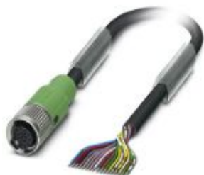
Sensor/actuator cable, 17-position, PUR halogen-free, black RAL 9005, free cable end, on Socket straight M12 SPEEDCON, coding: A, cable length: 5 m
