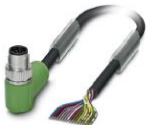
Sensor/actuator cable, 17-position, PUR halogen-free, black RAL 9005, Plug angled M12 SPEEDCON, coding: A, on free cable end, cable length: 10 m
