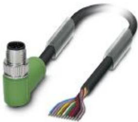
Sensor/actuator cable, 12-position, PUR halogen-free, black RAL 9005, Plug angled M12 SPEEDCON, coding: A, on free cable end, cable length: 10 m
