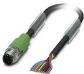
Sensor/actuator cable, 12-position, PUR halogen-free, black RAL 9005, Plug straight M12 SPEEDCON, coding: A, on free cable end, cable length: 3 m
